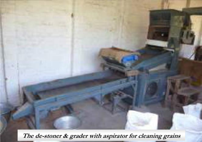
*The de-stoner & grader with aspirator for cleaning grains*
